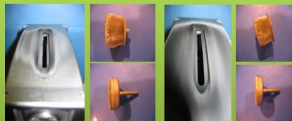
Heavy W growth on ion source without Xe/H 2
